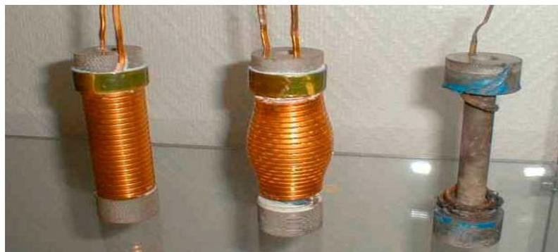
*Mini coils in different phases of testing. Left : original shape. Center : significant plastic deformation due to magnetic pulse. Right : Overloaded coil*
