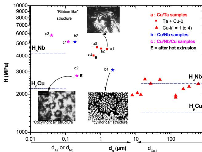
Plot of ultimate tensile strength of composite conductors vs. size of reinforcement component
