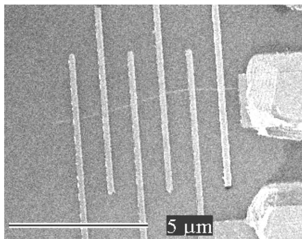
*SEM picture of CNT (horizontal) on contact array*
