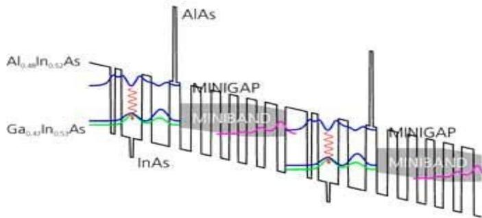
*Bandstructure of a quantum cascade laser.*
