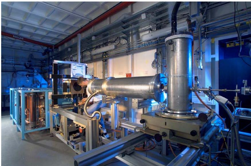
*Picture of mobile pulsed installation at ESRF. Far left, the generator, right of center the coil cryostat*
