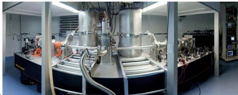
The principle of our experiment is to measure the ellipticity acquired by an incident linearly polarized light travelling in vacuum through an intense magnetic field region.
